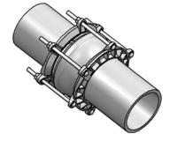
To ensure integrity of installation, wait 15 minutes, inspect for leaking, and confirm bolt torque. If necessary, retighten bolts evenly as required to stop the leak.
