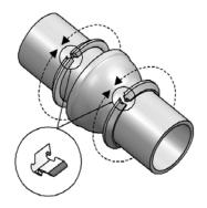
Interlock the ductile iron clamp ring segments on the spigot side of the joint. Ensure that the ductile iron clamp ring joint is rotated 90° (1/4 turn) from the gasket joint.
