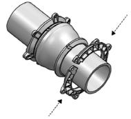
Hand tighten the nuts and ensure the ductile iron spigot ring is centered on the pipe and is making full contact with the face of the gasket. Tighten the nuts evenly until the spigot gasket compresses against the joint and the leak stops. Tighten nuts to approximately 20 - 30 ft. lbs. of torque.
