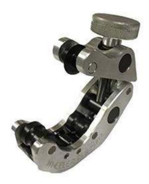
Designed for plumbing remodeling, commercial boiler and air conditioning jobs, where standard cutters simply don't have the room. Cuts thin-wall material like traps and tailpieces with no distortion. Good for under vanities, close to walls, waste and overflows. Eliminates sawing which can loosen joints. One cutter wheel (No. 8038) cuts both plastic and non-ferrous materials. For ½ to 2-3/8" (6-59mm) O.D. non-ferrous tube and plastic pipe and tube. Shipping weight....1.5lbs.
