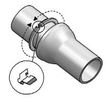
Interlock the ductile iron clamp ring segments on the spigot side of the joint. Ensure that the ductile iron clamp ring joint is rotated 90° (1/4 turn) from the gasket joint.
